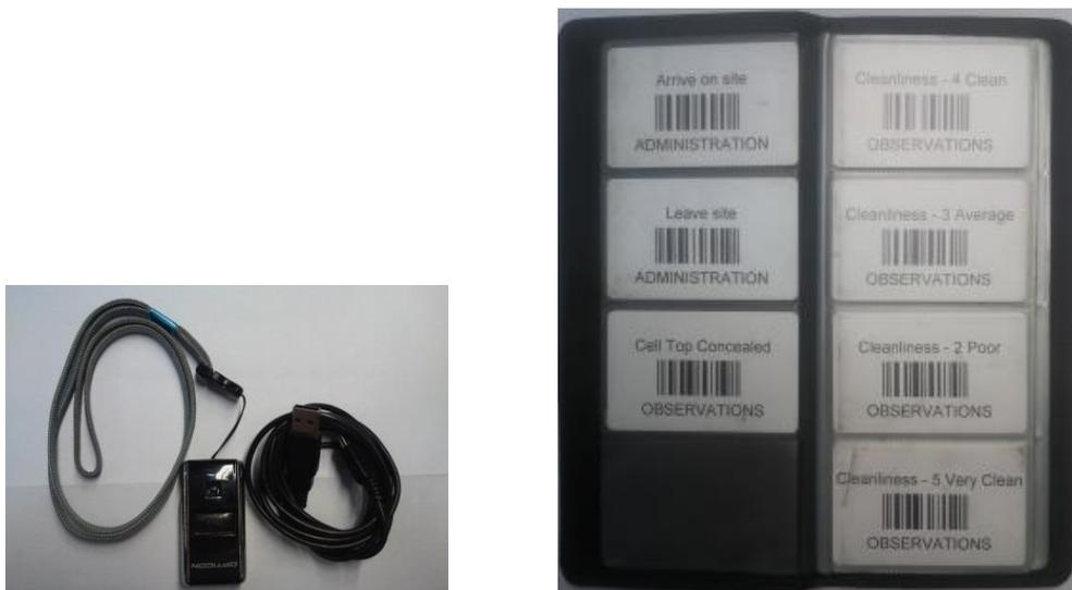
3. When performing a service, making an observation or repairing a battery the technician **scans the battery tag**, and then **scans the activity** contained in the activity code book (i.e. if you top a battery, scan "battery topped")
