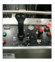
The Power Changer is operated from the easy to use joystick controls, and is powered from an overhead pickup rail. With two compartments, the Power Changer™ Series lets you make the maximum use of your rack space while operators remove and replace batteries quickly and efficiently.
