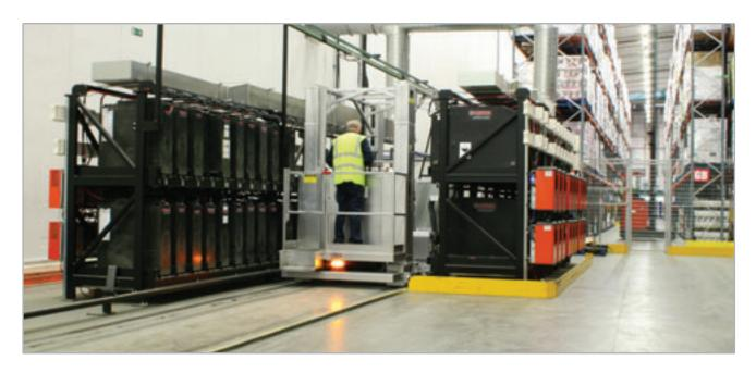
The Power Changer is an electrical driven battery transfer car that utilises a separate hydraulic power system for its lift, and operation of the transfer arm. By separating the drive and lift systems a lifting speed of 8 metres per minute and travel speed of up to 80 metre per minute can be achieved. This is one reason why the Power Changer is among the most efficient machines on the market today.
