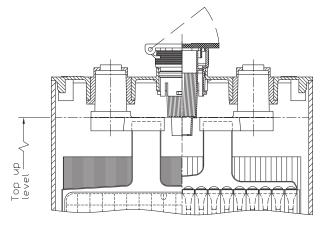
Do not fill the battery with electrolyte. The electrolyte level must not fall below the anti-surge baffle or the top of the separator.
